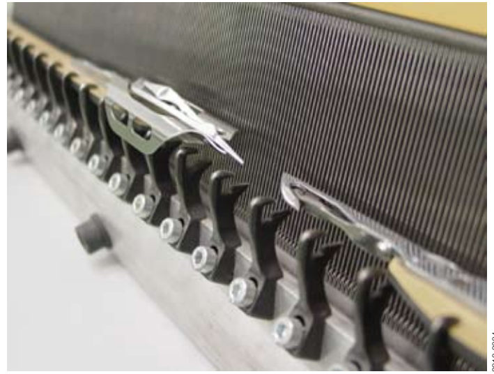
Precise rapier heads insert a broad range of weft yarns.
