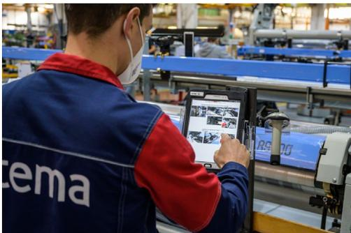
A phase of the manufacturing of the Iteima weaving machines in the Colzate plant. The operators, through tablets and scanners, have all the data of the machine assembly according to the principles of industry 4.0
