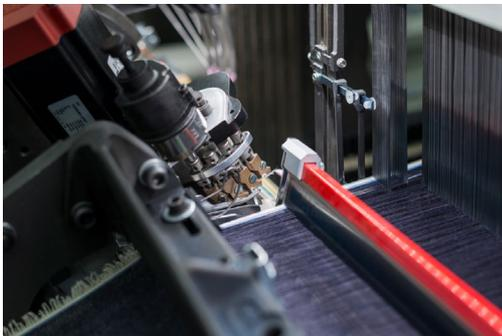
The breakthrough mechatronic device iSAVER® developed by Itemalab in 2018 that allows weavers to save up to 1.000 Kg of cotton thus establishing a new benchmark in sustainable weaving.
